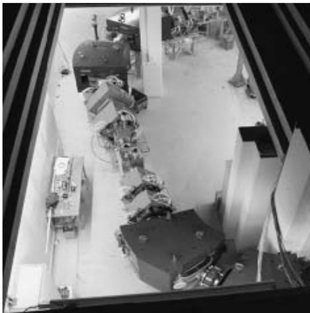
**Figure 2.** Photograph of the separator before closing the roof of its cave. The dipole sections consist of two dipole magnets each. Focusing is provided by quadrupole duplets. Between both sections a vacuum chamber is located that houses diagnostic elements and in the gas filled mode also the target.
