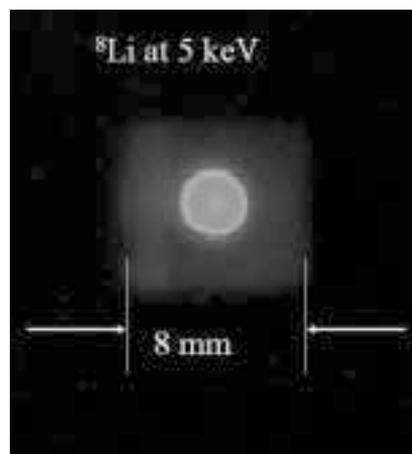
**Figure 3.**  $^8\text{Li}$  beamspot image from a small scintillator in the high field spectrometer observed with a CCD camera. More than 95% of the beam is estimated to fall within a 4 mm diameter.
