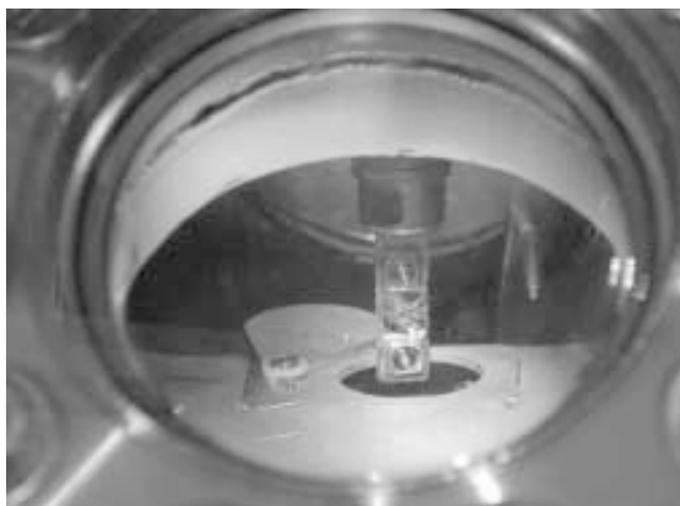
**Figure 5.** Photograph of the spectrometer on the high voltage platform. The bellows has been extended so that the sample and cryostat is in the loading position.
