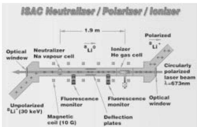
**Figure 2.** A schematic of the ISAC polarizer. A 30 keV  $^8\text{Li}^+$  ion beam is neutralized in the Na cell and then reionized in the He cell. In the intermediate drift region, a dye laser is used to pump the  $D_1$  optical transition of the  $^8\text{Li}$  atom with circularly polarized light. The resulting polarized ion beam is guided to either the  $\beta$ -NQR spectrometer or the high field  $\beta$ -NMR spectrometer
