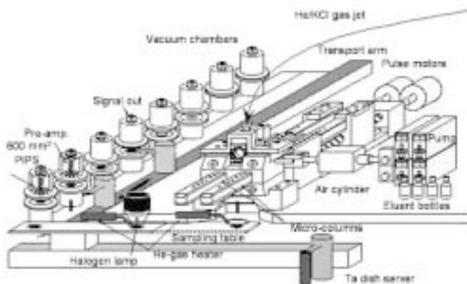
**Figure 4.** Schematic of the Automatic Ion exchange separation apparatus coupled with the Detection System for Alpha Spectroscopy (AIDA) [27].
