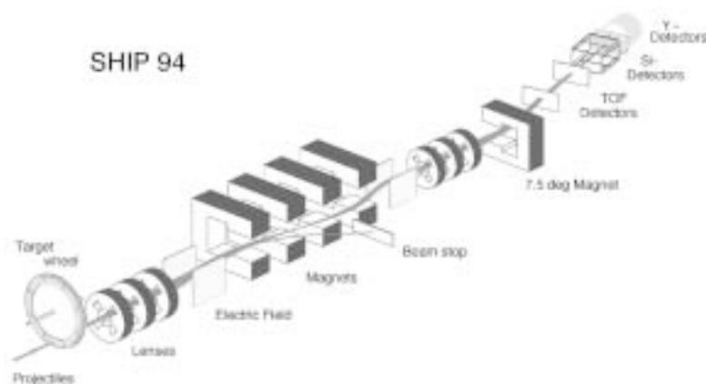
**Figure 2.** The velocity filter SHIP (Separator for Heavy Ion reaction Products) and its detection system. For details of the set-up see Ref. [2–4].
