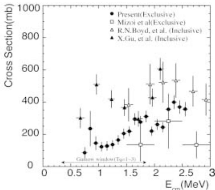
**Figure 2.** The reaction cross section of the  ${}^8\text{Li}(\alpha, n){}^{11}\text{B}$ . The open and solid triangles show previous inclusive measurements [5,6], whereas the open squares are the previous exclusive ones [7].
