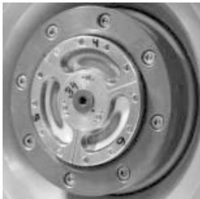
**Figure 3.** The GSI rotating target wheel.
