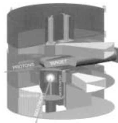
**Figure 1(a).** 3D view of the target, moderator, and reflector assembly.
